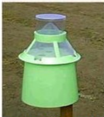
Boll Weevil Trap These traps are specifically designed for monitoring and mass trapping cotton boll weevil
